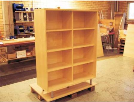
Start with a loose shelf in the ninth hole from the bottom, then a fixed shelf in the 20th hole. (One shelf in each back joint). Lock the shelves. Fixed shelf should be screwed on with system screw FX 6,3x10 Fzb.
