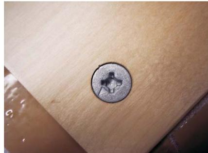
Press the worm minifix diam. 15/19 fzb, into the sides and middle side, 6 in each. The arrow
