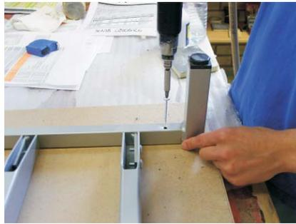
Appliance bag 61167423 should be used. Put out the middle frames, assemble the plinth gable on the middle frame with screw M6x16. Put the complete leg frame on the bottom, first screw on the plinth gables with screw 5,0x45 in the predrilled holes, then use screw 4,5x25 in the small mounting rings on the middle frame.
