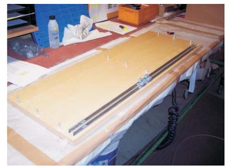
One end stop in each end of the rail. Two trolleys in each rail, should be turned according to picture.
