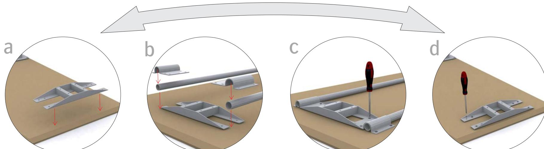
a Assemble the table holds in the predrilled holes with screw A (10 screws per gable).
